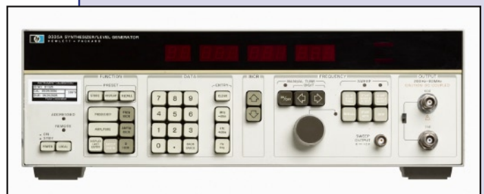
HP 3335A RF cal lab work-horse
